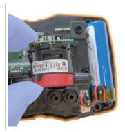
Remove hose connections from the faulty sensor/bridge.
