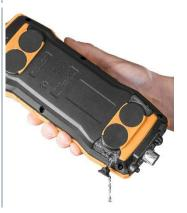
Wipe off any drops still on the condensate outlet with a cloth and close the condensate outlet.
