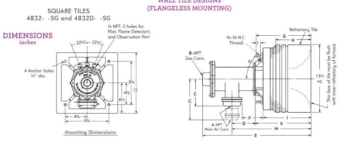
Standard 131/2" square tile shown. For dimensions of optional round or tapered tiles, see below or page 2. All standard tiles are grooved for better resistance to fluing.
