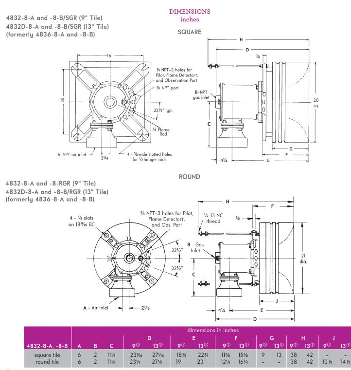
† Detector must be located "downstream" of pilot in regard to main air spin (see Bulletin 4832).
