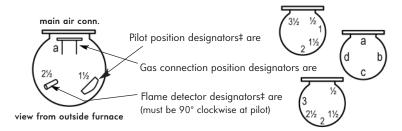
Arrangement Designators are specified relative to the main air connection at 12 o'clock and should be listed for pilot, gas connection, and flame detector in that order.
