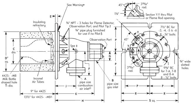
NOTE: For 4425-8-A, the air and gas connections cannot be piped in the same plane, as shown on other side, because the "flower pot" type air connection flange would interfere with the 2½" gas line.
