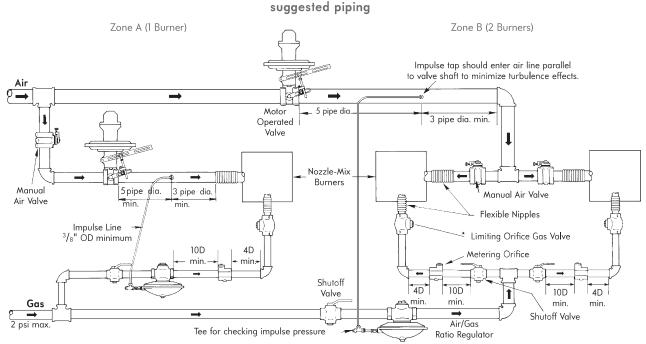
\* Limiting orifice gas valves must be mounted as close to the burner as possible
