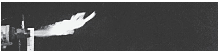
1¼" 4020-LP Nozzle-Mix Pilot Tip 100% excess fuel 0.1 osi air pressure
