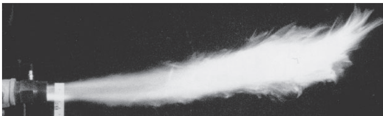
2½" 4020-HP Nozzle-Mix Pilot Tip 100% excess fuel 8 osi air pressure
