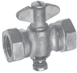
1808-01 Gas Shutoff Cock (½" FNPT, brass) for gas up to 0.5 psi. A plug in the handle conceals a port adjustment for setting flow through valve. Used as pilot gas cocks on 4988 Burners.
