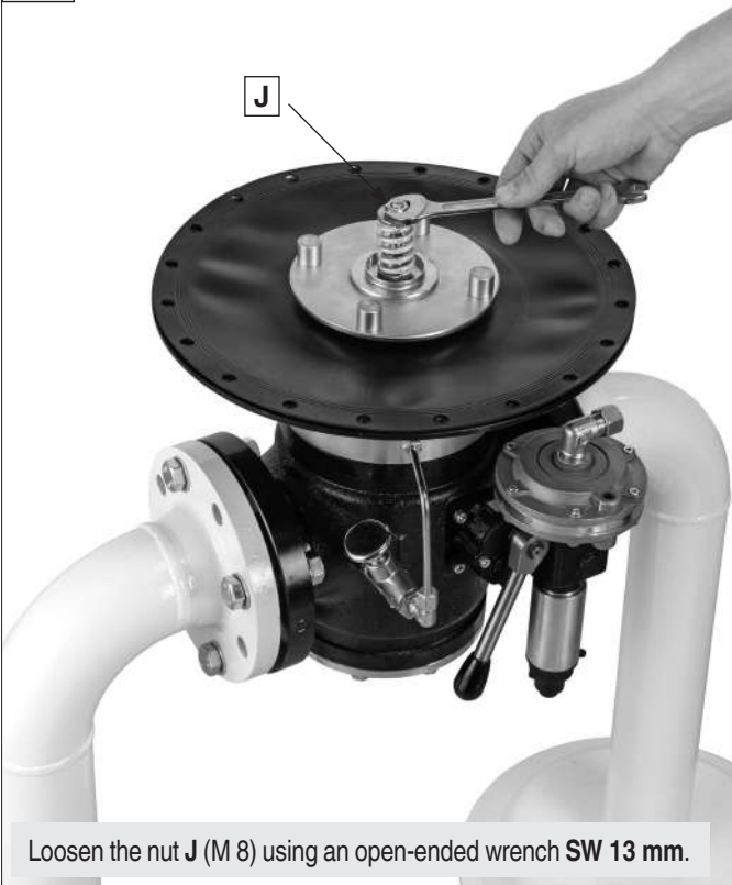
Loosen the nut J (M 8) using an open-ended wrench SW 13 mm .
