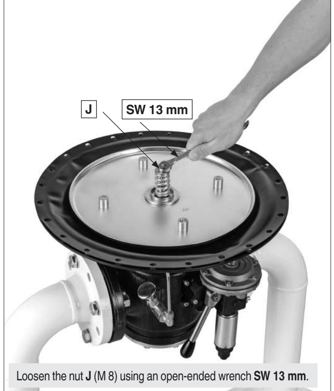
Loosen the nut J (M 8) using an open-ended wrench SW 13 mm .
